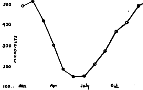
FIG. 9. SEASONAL TREND OF RADIO FIELD STRENGTHS (NIGHT) OF WBBM (770 KC.) AS RECEIVED AT BOSTON. VALUES HERE REPRESENTED ARE ST CORRECTED FOR TWILIGHT EFFECT; WHICH DEPENDS UPON ANGLE OF DEPRESSION OF THE SUN BELOW THE HORIZON DURING PERIODS OF OBSERVATION.
